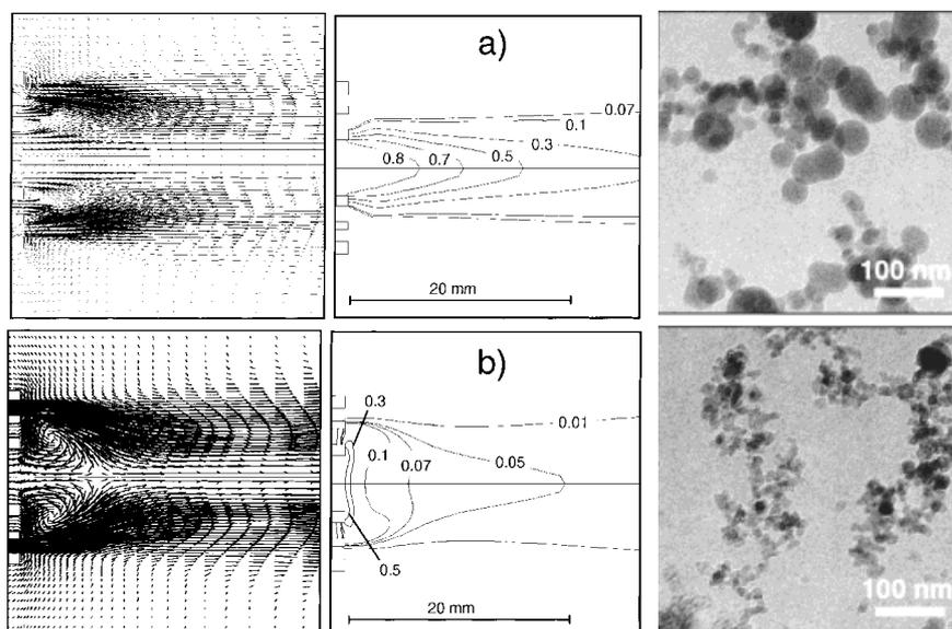
**Figure 12.** Velocity vectors (right), iso-molar lines of argon fraction (middle), both calculated by computational fluid dynamics, and TEM micrographs of  $\text{SiO}_2$  product powder (right), obtained from a micro scale diffusion flame reactor [8]. The flow rate of oxygen through the third (outer) tube is 1.5 L/min (a) and 8 L/min (b), while the flow rates of argon (center tube) and methane (second tube) were kept constant 0.25 and 0.4 L/min, respectively (courtesy of K. Wegner, ETHZ).
