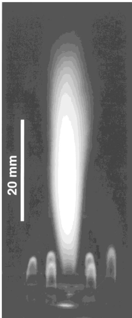
**Figure 9.** Self-sustaining spray flame, making fumed silica from a 0.1 molar HMDSO in an ethanol solution.
