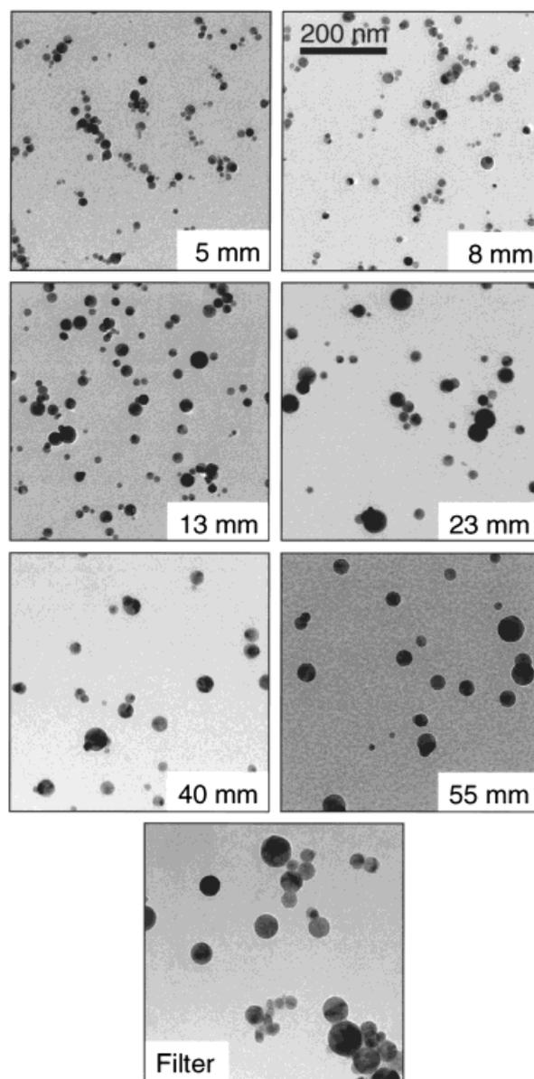
**Figure 5.** TEM pictures of TiO<sub>2</sub> particles at increasing heights above the burner as obtained by thermophoretic sampling in a premixed TTIP/methane/oxygen flat flame.
