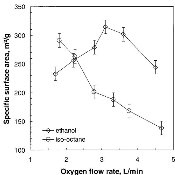
**Figure 11.** Specific surface area of  $\text{SiO}_2$  particles made by FSP for 0.1 molar HMDSO/organic fuel solution as a function of dispersion gas (oxygen) flow rate using ethanol (diamonds) and iso-octane (circles) as solvent.
