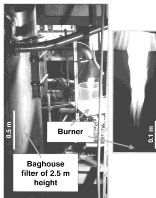
**Figure 7.** Photograph of a pilot-scale flame aerosol reactor, which can produce nanostructured silica-carbon powders at production rates up to 700 g/h.
