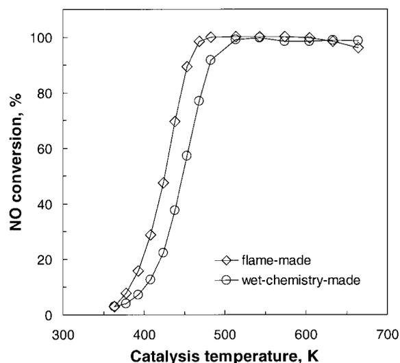
Figure 6. NO-conversion as a function of catalysis temperature for a flame-made (diamonds) and wet-chemistry-made (circles) vanadia coated titania catalyst (courtesy of W. J. Stark, ETHZ).
