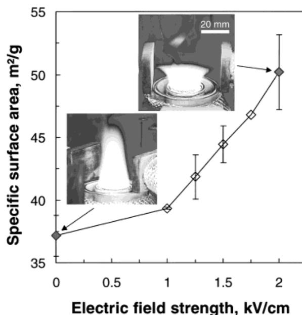
**Figure 3.** Specific surface area of the  $\text{TiO}_2$  product powder made by titanium tetraisopropoxide (TTIP) oxidation in a premixed methane/oxygen flat flame as a function of the applied electric field strength.
