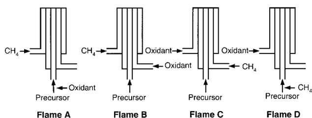
**Figure 2.** Reactant mixing configurations for a double or inverted (Flame A and B) and single or classic (Flame C and D) diffusion flame reactor [2].
