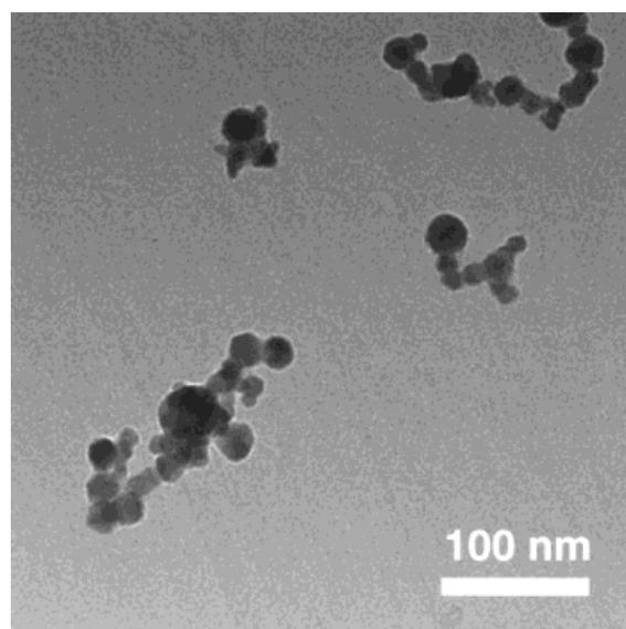
**Figure 10.** Transmission electron micrograph of  $\text{Bi}_2\text{O}_3$  particles made directly by flame spray pyrolysis (FSP).
