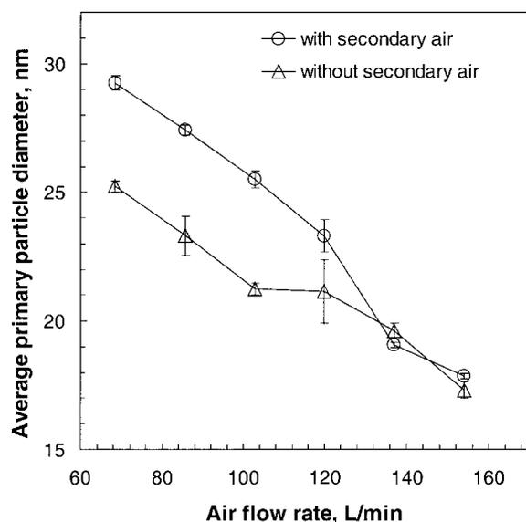
**Figure 8.** Average primary particle diameter obtained by nitrogen adsorption (BET) as a function of airflow rate with (circles) and without (triangles) secondary air entrainment at production rates of 300 g/h in the reactor of Figure 7.
