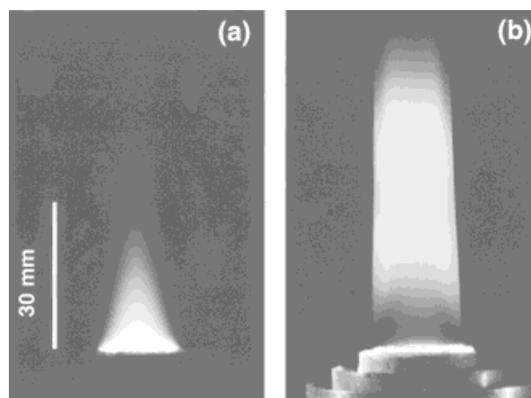
**Figure 1.** Premixed hexamethyldisiloxane (HMDSO)/methane/oxygen flat flame: (a) in the absence and (b) in the presence of a laser sheet.
