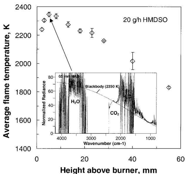
**Figure 4.** Axial temperature profile of a premixed HMDSO/methane/oxygen flat flame. In the lower part of the figure a typical comparison of the normalized radiance spectrum with the blackbody Planck function is shown, using a least squares fit at the wavenumber range of hot CO<sub>2</sub> (2200–2300 cm<sup>-1</sup>). Species detectable at other wavenumber ranges are named.
